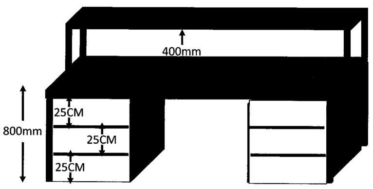
We included a raised platform at the end half of the table to accommodate decanting of water samples. We prefer Epoxy resin as the lab table top material for durability, chemical resistance, bacteria resistance, and easy-to-clean surface.
